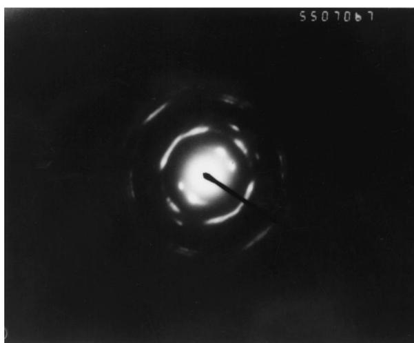
Figure 7 SAED pattern of the fiber shown in Fig. 6.
